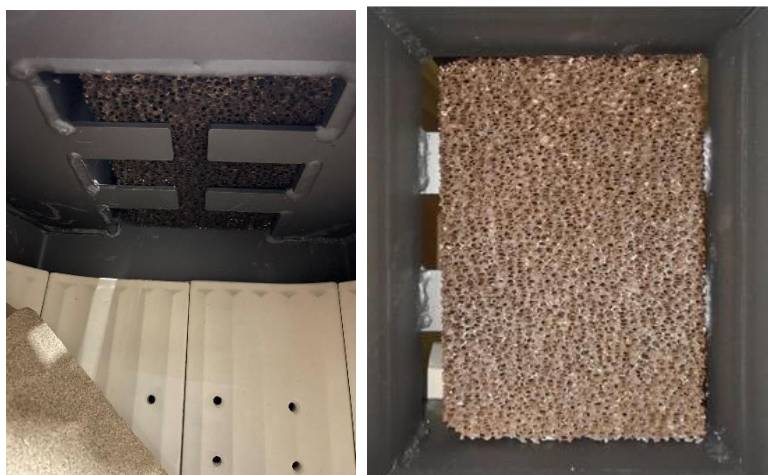
Katalysatormontage over kuglefanget bag røgvenderen for M, Maestro, QM40 ecoline
