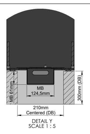
**MB: Manuel Burner** DB: Electrical burner (Denver Basic)
