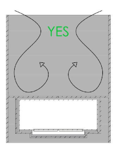
DO! install the fireplace in an open-wall construction, which is closed above and below the fireplace. Make sure to create a closed cavity for the section below the base plate of the fire.
