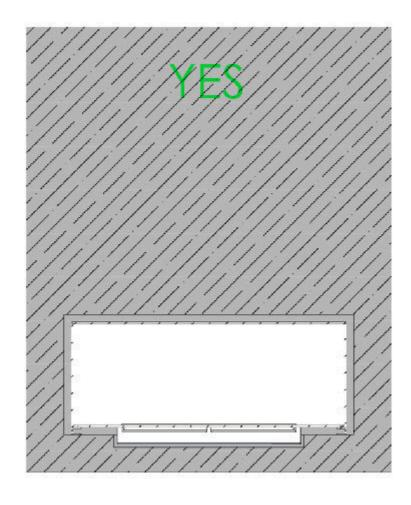
DO! install the fireplace in a massive wall (made of bricks, stone or gas beton) using the wall cut-out dimensions mentioned on the previous page.
